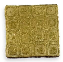
Plain mica has no color. But when metal oxides, such as titanium dioxide, iron oxide, silicon dioxide, or tin oxide are applied to the mica, it can take on a color. By changing the metal oxide used, and the thickness of the layer, mica powder can be manufactured to appear to be pearl, white, gold, silver, copper, or bronze color. By adding other metal oxides, other colors can be achieved like blue, green, or red.
